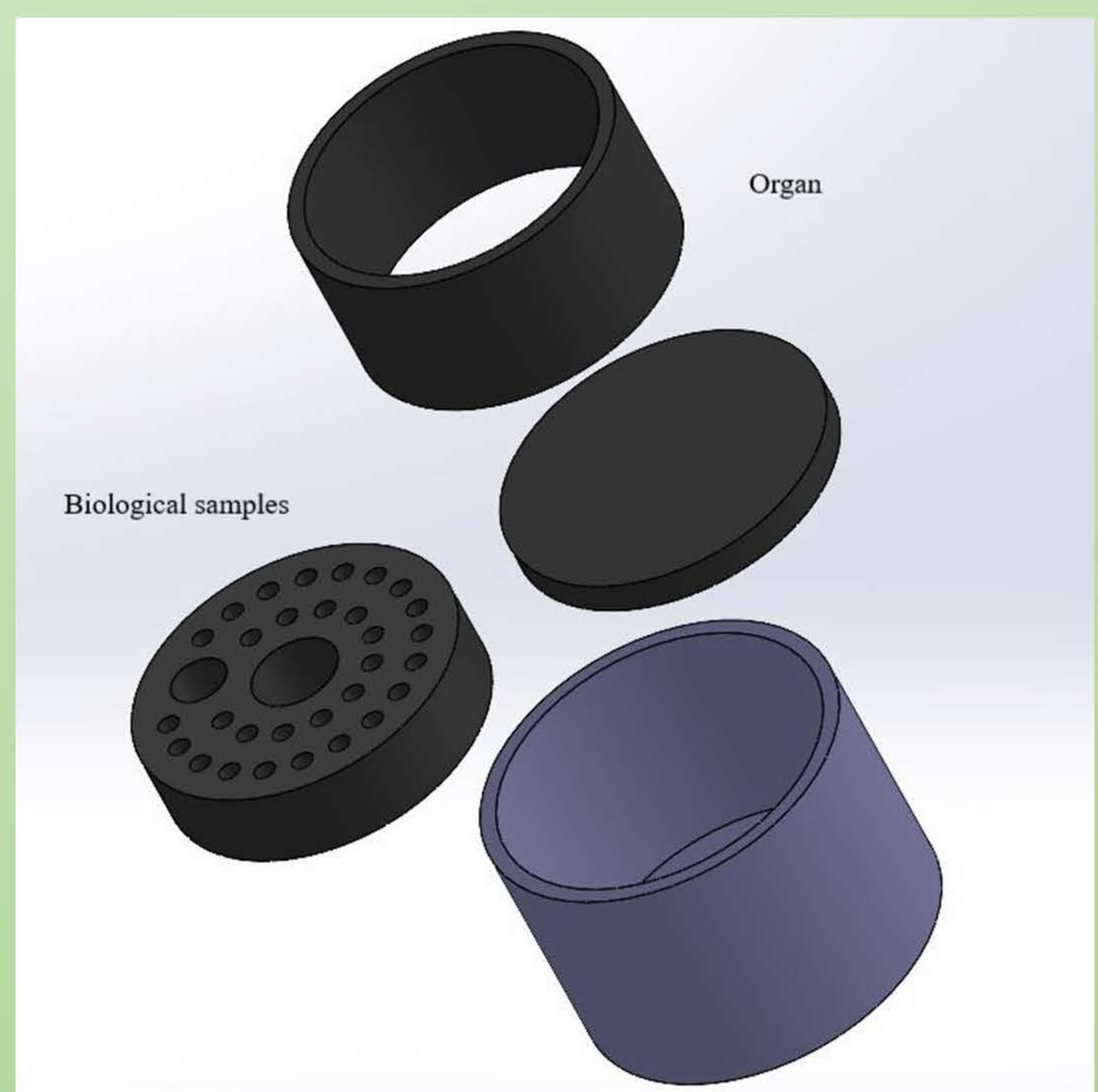
Figure 1 The figure shows the configuration of the primary container and of the foam rubber (shock-absorbing) platforms
